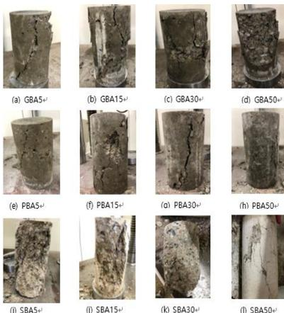
Fig. 5 Failure Mode of Specimen
